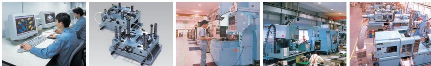
● Design with 3-D CAD ● Manufacturing of metal molding parts ● Electrical discharge machine ● Machining Center ● Injection molding machines
